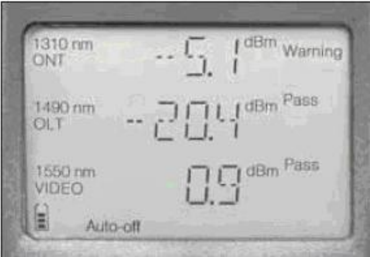
Figure 4-4 Measurement interface of the optical power meter
