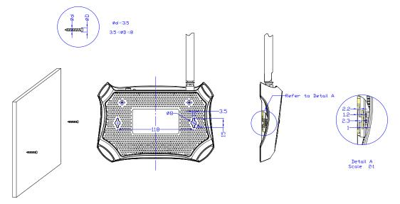
Figure 2-3 Wall-mount Install
