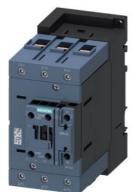
power contactor, AC-3e/AC-3, 110 A, 55 kW / 400 V, 3-pole, 230 V AC, 50 Hz, auxiliary contacts: 1 NO + 1 NC, screw terminal, size: S3, upright mounting position
